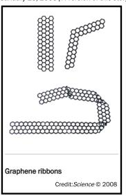
YING TOGETHER materials science and chemistry, scientists have developed a chemical method for making carbon ribbons less than 10 nm wide and just one atom thick (*Science*, DOI: 10.1126/science.1150878). The semiconducting properties of these so-called graphene nanoribbons make them promising materials for electronics applications.
